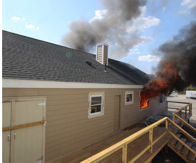
Figure 5.10: Photograph of exterior fire conditions at bedroom 3 window 90 s after window ventilation during Experiment 4.
