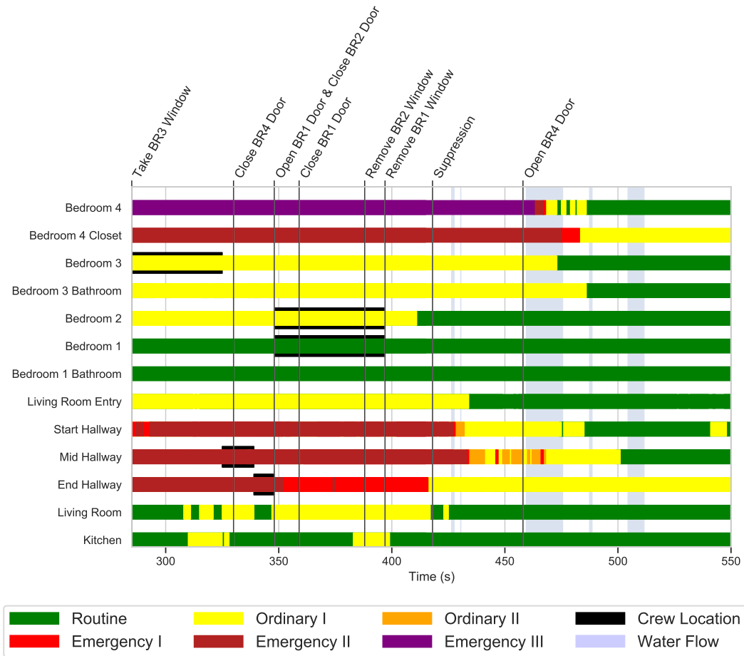
Figure 5.19: Thermal operating conditions based upon 3 ft elevation temperatures and heat fluxes during post-intervention period for pre-suppression search tactics in Experiment 8.
