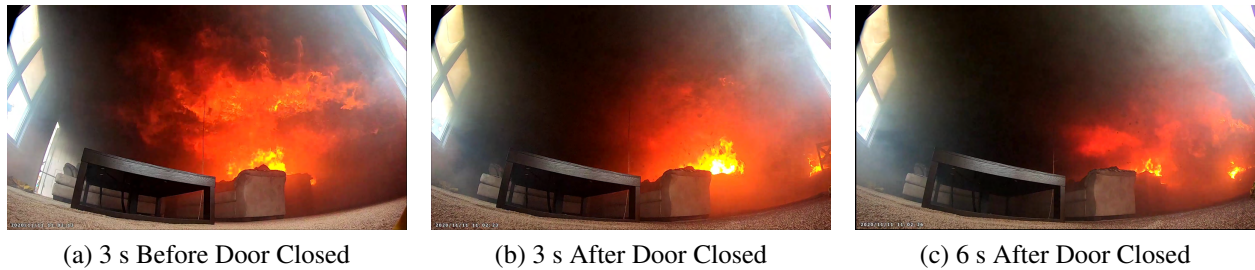
Figure 5.21: Fire conditions preceding and following front door closure during Experiment 16.
