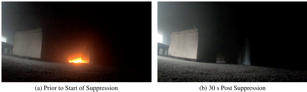
Figure 5.32: Images looking from the living room toward the hallway showing smoke layer height in Experiment 2 prior to suppression and post suppression.
