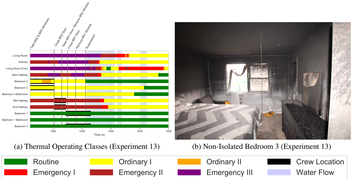
Figure 5.27: Thermal operating conditions during Experiment 13 based upon 3 ft elevation temperatures and heat fluxes during post-intervention period for pre-suppression window initiated search tactics (left). Post experiment photographs of bedroom 3 (right).
