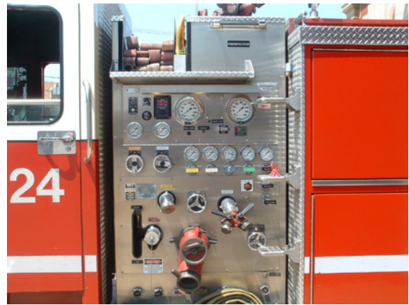
This crosslay is a static hosebed designed to accommodate up to 400 feet of hose. Note the "wye" connected to the outlet. Another "wye" is on the officer side of the engine.
